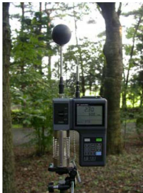
Figure 4. Measurement of air temperature / relative humidity / wind velocity / radiant heat.
